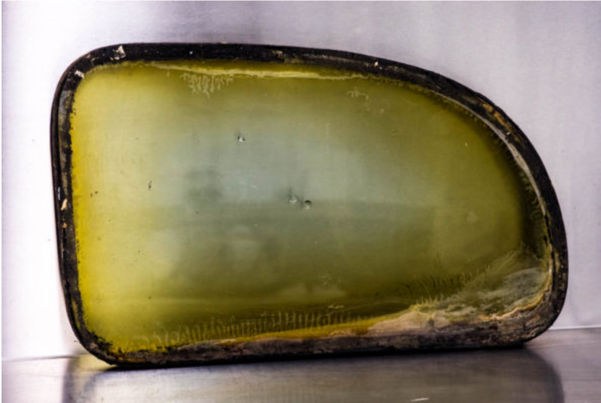
Bullet proof rear window, passenger side, reflecting remains of the dashboard.
