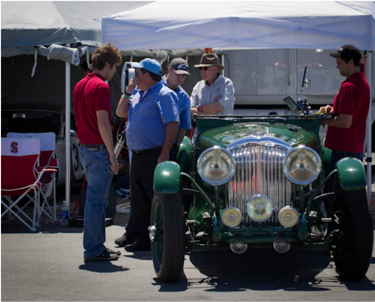
Preparing the Eddie Hall Bentley – car instrumented to record performance variables
