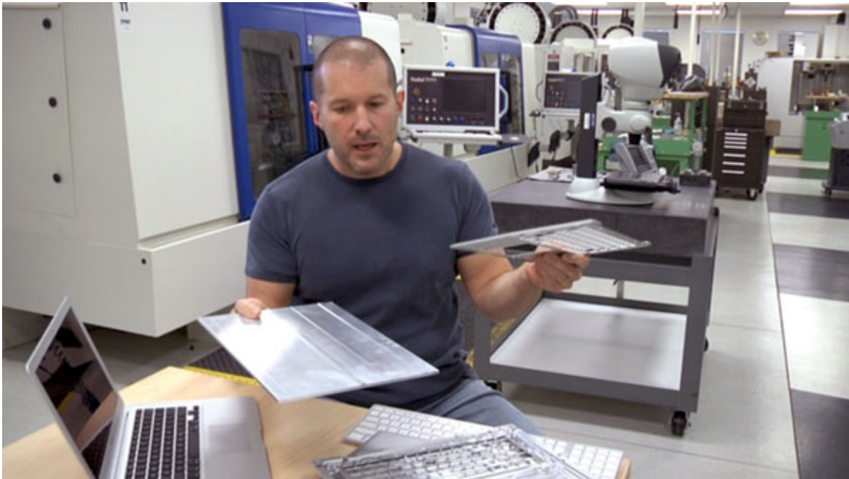
Jonathan Ive, of Apple, describes how the aluminium pressing at the heart of the Macbook Air is not so much an artifact as a process – articulating different key stages and components of manufacture as well as the other components of the laptop.
